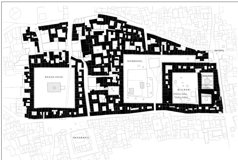
Figure 6: Nagbahal, Patan. The area exhibits an example of planned residential settlement with large open quadrangles with community facilities. (Pant and Funo 2007)
